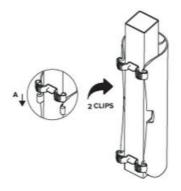
Using closed-tube clips for tubular uprights Slide clip over the hooks on the guard (A). Repeat process for second clip.
