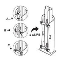
Using standard clips for openback uprights Insert first clip into the back of the post (A). Turn the clip 90° (B) and slide the clip over the hooks on the guard (C). Repeat process for second clip.
