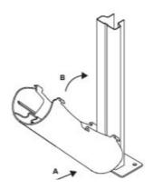
Slip base of guard onto upright (A) then pivot top of guard into place (B).
